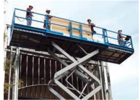
Scissors Lift: Wide work platform
